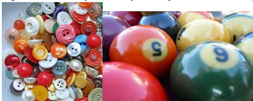
Figure 6.3: Materials made by bakelite polymers, formaldehyde is used as monomers in production of bakelite polymers.
